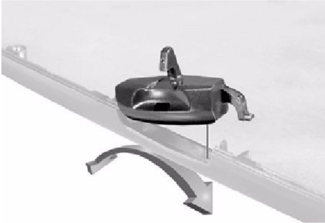
3. Remove the [display assembly bezel](#).
