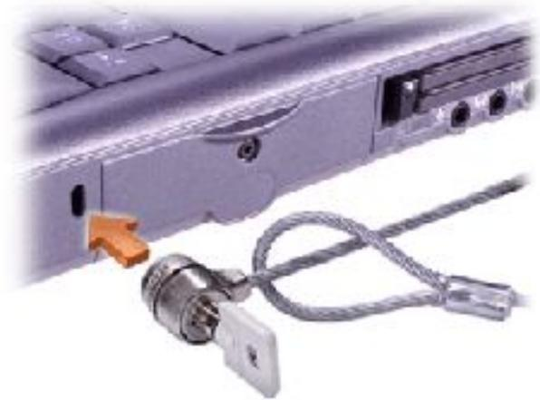
The slots (one on each side of the computer) let you attach a commercially available antitheft device to the computer. Complete instructions for installing antitheft devices are usually included with the device.
