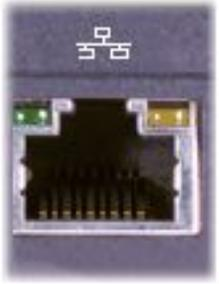
If you ordered the optional integrated network adapter, use this connector to connect the computer to a network. If a network cable is connected to the network connector, the green light indicates that the network connection is active. If you do not see a green light after connecting a network cable, try replacing the network cable. An amber light indicates that the network adapter driver is loaded and the adapter is detecting activity.
