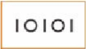
Use this connector to attach a serial device, such as a palmtop, to the computer.
