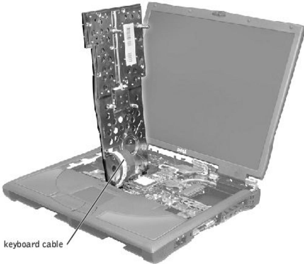
7. Disconnect the keyboard cable and lay the keyboard assembly aside.
