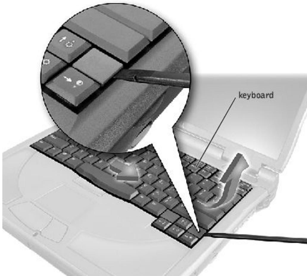
5. Lift the right end of the keyboard, and slide it slightly to the right to disengage the tabs at the left end.
